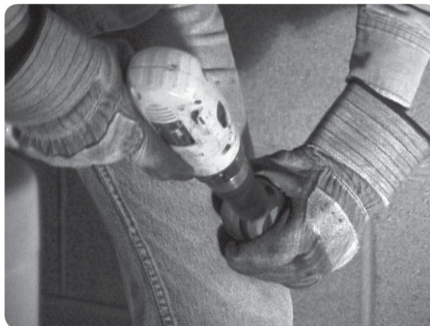
Solution: Using wire brush with power driver
