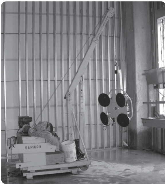
Power vacuum lifter avoids manual lifting
